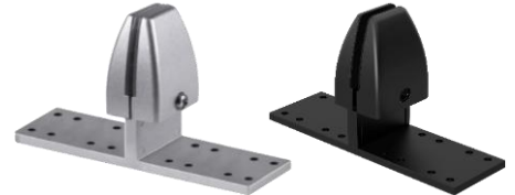
SBUDUALSI 5 3/4" wide x 1 3/4" deep x 3 1/2" high For use mounting panel above two shared worksurface. Installs between two 1" thick work surface
